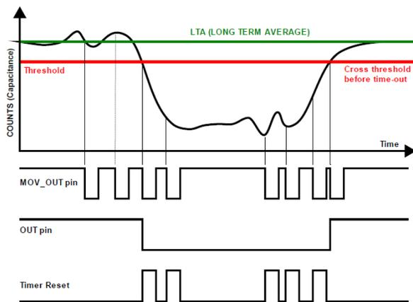
Figure 2: Plot of IQS229 streaming data along with the digital response
