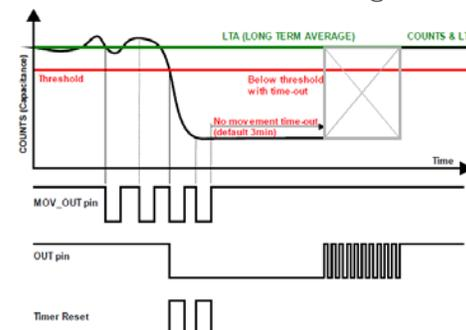
Figure 3: Example of a time-out with re-calibration
