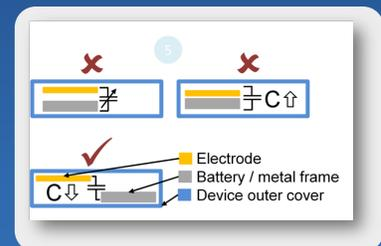
Avoid placing the electrode near large conductive areas as this may cause significant changes in capacitance or decrease sensitivity.
