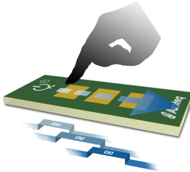
Figure 1: Example of a 3-channel sense electrode for a swipe-switch device.
