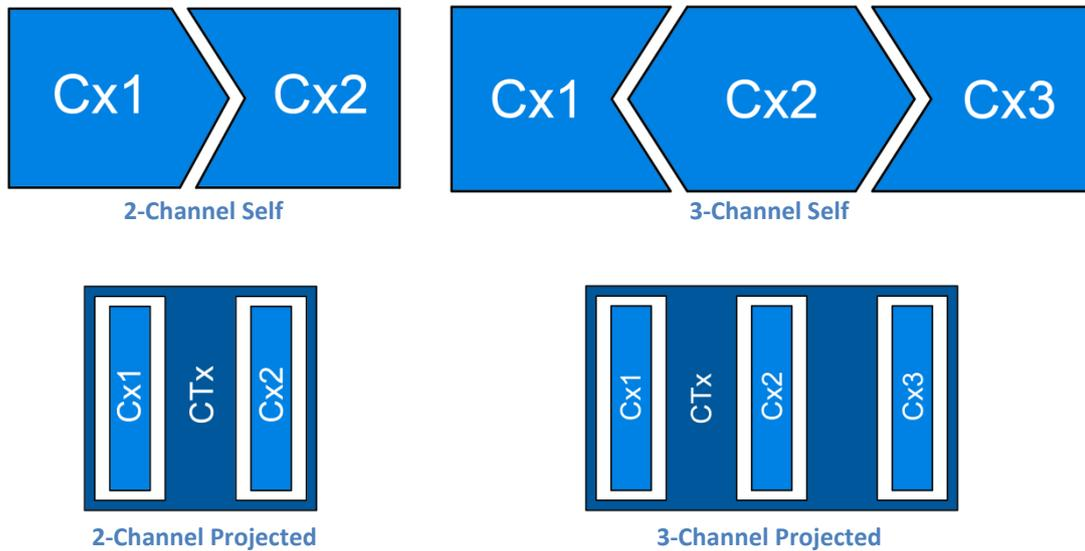
Figure 2: Example sense electrodes.
